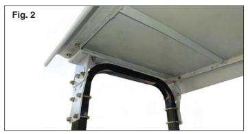
This canopy and its mounting hardware was carefully designed to fit a wide variety of ROPS. While most of the pieces will be self explanatory, a few pointers can help clarify the desired end result. See Fig 1 and 2.
